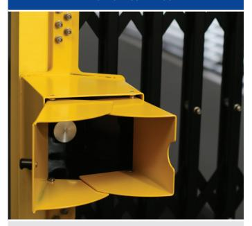
• Uniquely designed emergency escape locking system. Allows for opening of the door in emergencies without the need of a key. The box that houses the keyless lock has been designed so that it can only be accessed from the inside. The locking mechanism is further protected by steel lockstile protector plates and an anti-drill disc.
